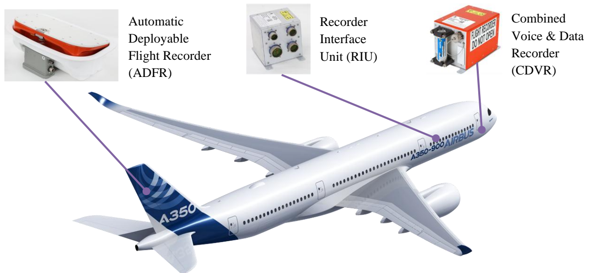
Flight recorder installation on Airbus A350 (Credit: Leonardo and Airbus)
